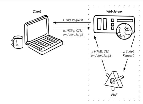
FIGURE 1.7 PHP can dynamically generate HTML, CSS, and JavaScript on the Web server, which is then sent to the browser.
